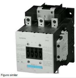
CONTACTOR, 90KW/400V/AC-3, AC(40...60HZ)/DC OPERATION UC 23...26V AUXIL. CONTACTS 2NO+2NC 3-POLE, SIZE S6 BAR CONNECTIONS CONVENT. OPERATING MECHANSIM SCREW TERMINAL
